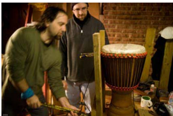
Step 6--Begin high tensioning with rope puller (they don't use these in Africa)
