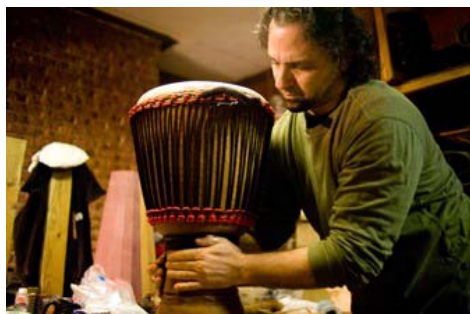
Step 8--wrap the excess rope (used to tune the drum later)
