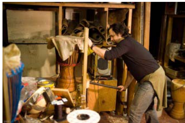
Step 5--begin tensioning the vertical ropes, trim excess goat skin
