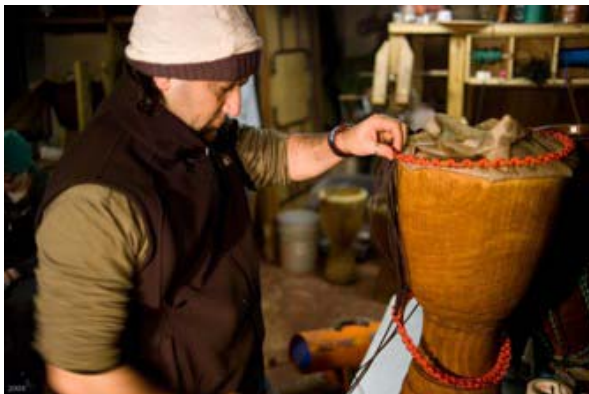
Step 3--tie knots around the rings to hold the "vertical" ropes
