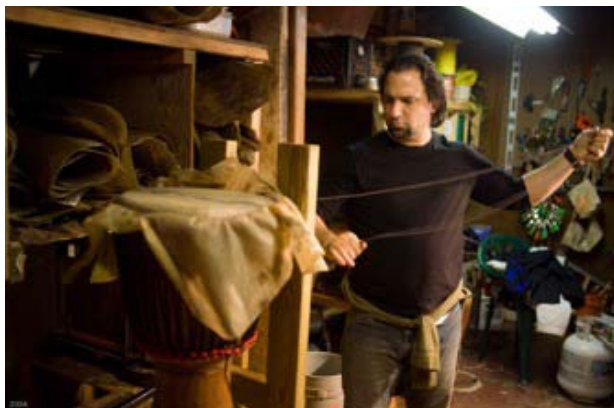
Step 4--fit the goat skin on the drum & string the vertical ropes
